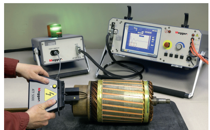
Testing an armature using the ZTX accessory and the ATF5000 commutator probe.
