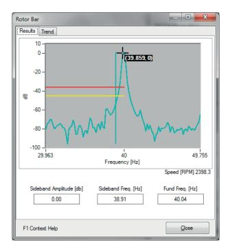
The EXP4000's rotor bar spectrum analysis graph.
