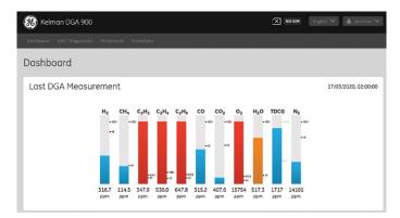
This facilitated operational decisions without needing to go to site for manual oil sampling. It avoided unplanned outages, increased network reliability and enabled the move to condition-based maintenance.
