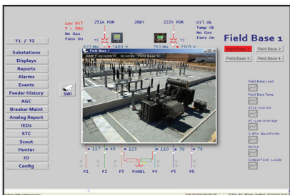
Live Video Feed Directly in a SCADA
