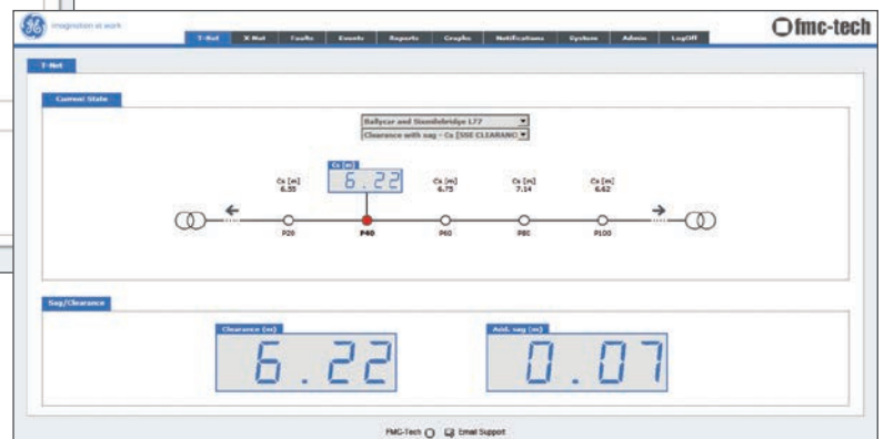
Application delivers site specific line sag and clearance for safety constraint verification and maximum line utilization
