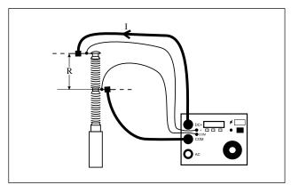
Measuring the resistance of a breaker
