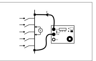
Measuring resistance at busbar joints
