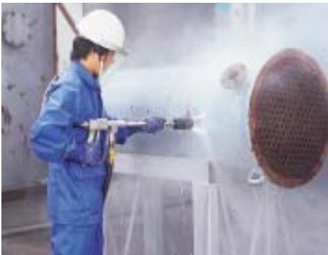
Outer surface cleaning of heat exchanger by Grip Jet Gun with V-Rotary Nozzle.
