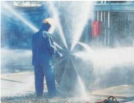
Cleaning of heat exchanger with Lance Nozzle.
