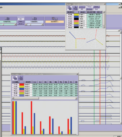
Analyze transformer faults using both analog and digital power system quantities that are measured and recorded up to a rate of 64 samples per cycle.
