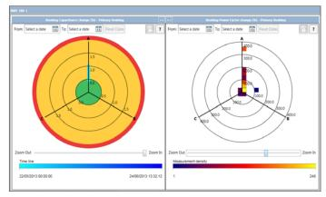
Bushing power factor and capacitance alarms
