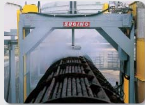
熱交換器の外側洗浄 Cleaning of Tubebundle Outside
