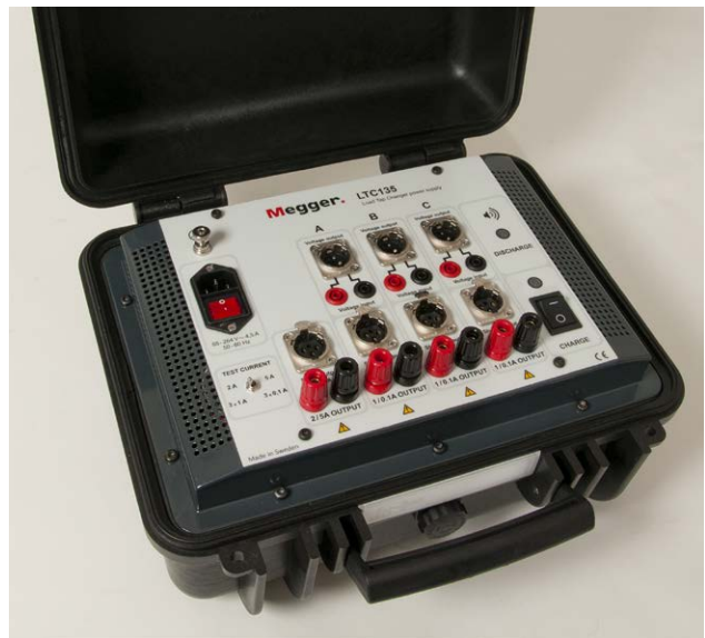
LTC135, Load Tap Changer power supply
