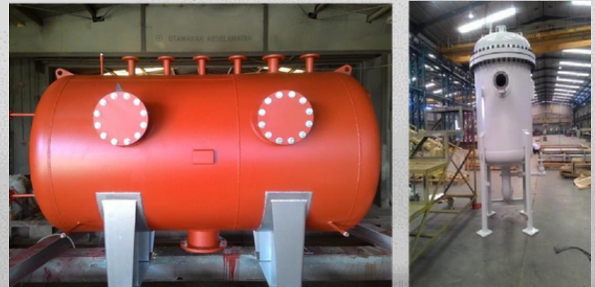
AMMONIA PLANT, CONDENSATE TANK
