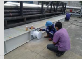
Welding Quality Test Penetrant Inspection & Magnetic Particle Inspection (MPI) Test
