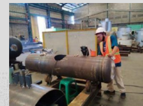
Welding Quality Test Penetrant Inspection & Magnetic Particle Inspection (MPI) Test
