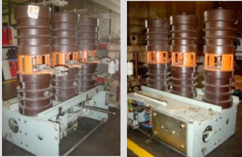
Retrofit VCB Mining - Sumatera
