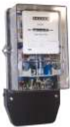
Energy meter 3P kWh Inductive Type Voltage 3x 220/380 V, Current .../5A or direct 5 (20) A
