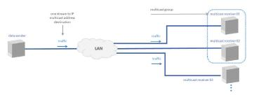
When it comes to power systems communication, IGMP protocol can be used when there is multicast communication between a Phasor Measurement Unit (PMU) and a Phasor Data Concentrator (PDC). With IGMP snooping, the receiver can send a "join group" to join an IP multicast group. To stop receiving data, the receiver sends a "leave group". Reason S20 has support to IGMPv1, IGMPv2 and IGMPv3 protocols.
