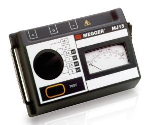
The BM15 and MJ15 are compact 5-kV insulation testers. They are very simple to use and provide a quick and accurate reading of insulation resistance. The instruments use an analog display with a maximum reading of 20 G $\Omega$ . The BM15 is powered by batteries. The MJ15 has an additional hand-cranked generator.
