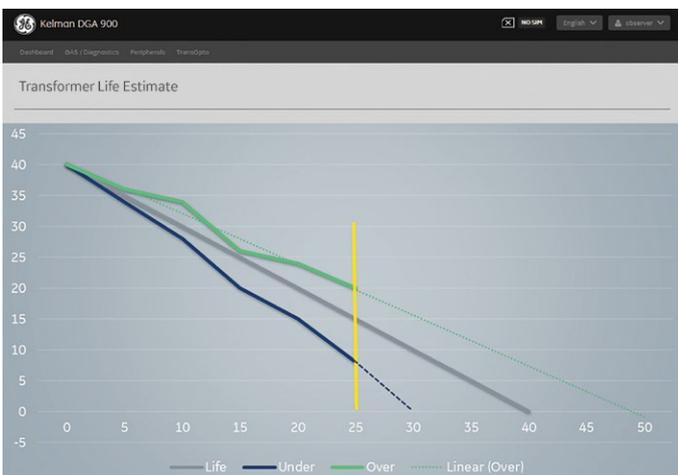
These models convert raw data into additional intelligent information to monitor the state of the transformer's insulating system every 10 minutes and determine its long term aging profile.
