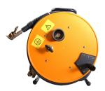
Portable high voltage cable reel with HV return, 18" high X 20" effective width with 130' of HV cable (shown here) and connectors 14mm MC connector compatible with T1 terminations (shown here); also available with 50' or 85' of HV cable and also for T4 and PFL terminations. For details check special data sheet for cable reels and racks
