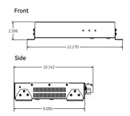
High Voltage Resister Box Module (Field Voltages 600 VDC - 800 VDC)
