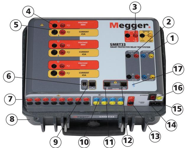
1. **Binary Outputs #1 and 2:** Rated for 300 V at 8 amps.
